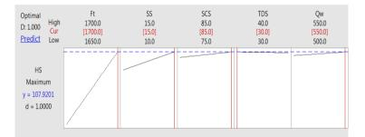
Fig.4 Optimization plot of Hardness Number Vs. Ft, SS, SCS, TDS and Qw
